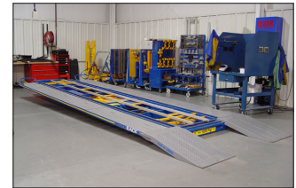
Figure 5—It is also necessary to ensure that the vehicle is properly stabilized when using other types of lifting equipment such as this bench rack.
