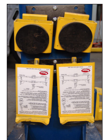
Figure 4—These auxiliary adapters, provided by the lift manufacturer, are specifically designed for the lift.
