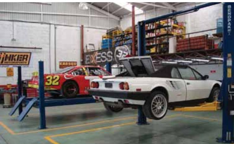
Lift purchase considerations include facility layout, types of vehicles to be worked on, accuracy and speed at which a vehicle can be properly positioned on the lift, kinds of services performed, ergonomics and worker safety and features that make the technician's job faster, more accurate and easier. Photo courtesy of BendPak
