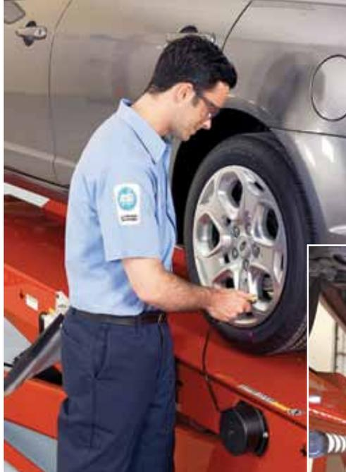
Numerous options and accessories are available for vehicle lifts, like these lighting and inflation stations, neither of which require additional or exposed electrical cords or hoses, which helps to keep the work area clear.
