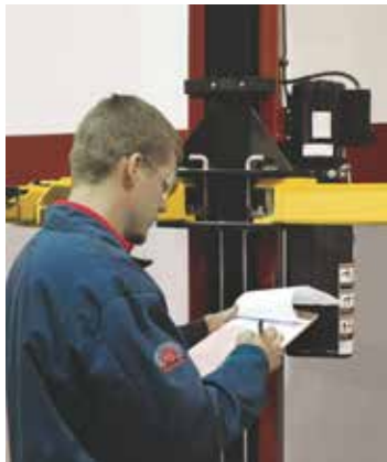
During a vehicle lift inspection, an ALI Certified Lift Inspector will evaluate the lift's operating mechanisms, safety systems, structural integrity, modifications and maintenance.
