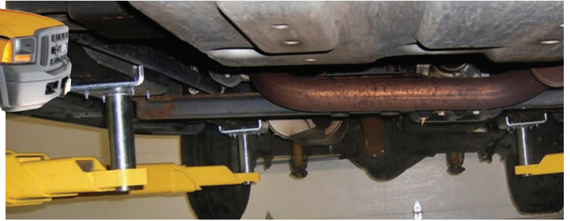
Frame-cradling adapters are recommended for two-post lifts.
